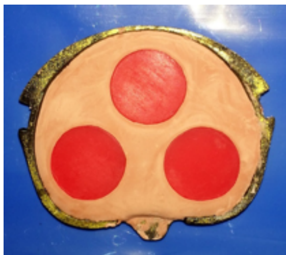
Figure 1. Wax pattern for porosity test
