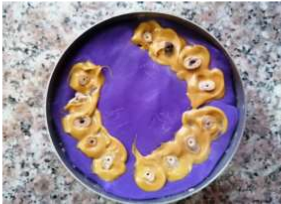
Figure 2: Roots imbedded in addition silicone material and covered with varnish
