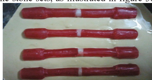
Figure 3: the waxed samples for tensile test embedded in the lower half of the flask.
