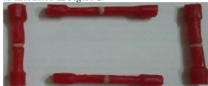
Figure 2: the wax blocks for acrylic teeth tensile test.
