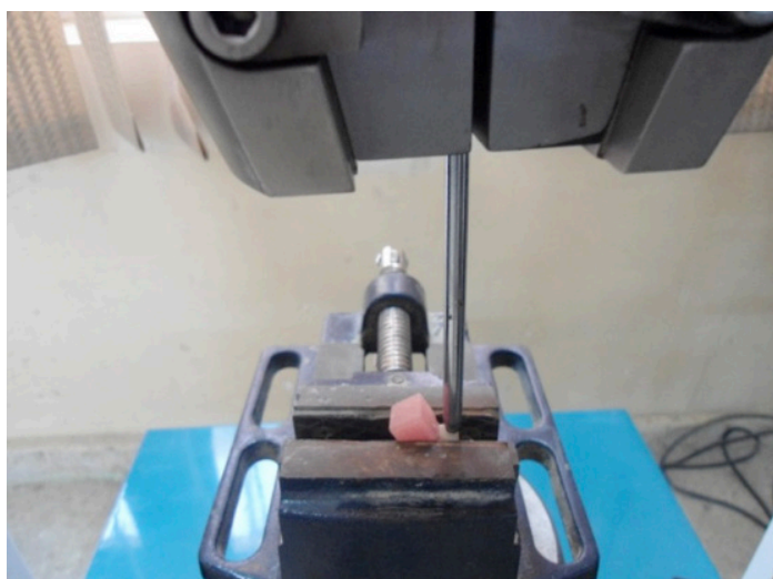
Figure (6): specimen with chucks in place ready for test.
