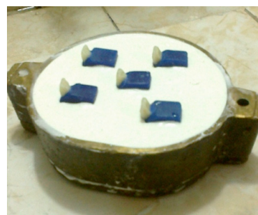
Figure (4): The wax pattern when insert in stone.
